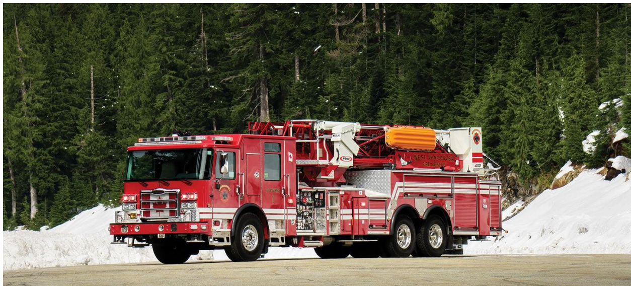
Figure 1: 100-foot Aerial Fire Truck
